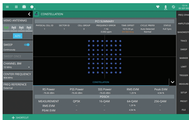
LTE Modulation Quality EVM Measurement on PBCH and PDSCH
