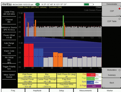
Modulation Quality – EVM High or Low Values will Create Larger Areas of Cell-to-Cell Interference and Create Lower Data Rates Near Cell Edges. Low Values Affect In-Building Coverage.
