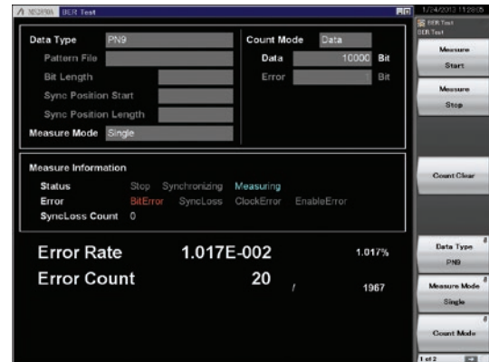
BER Measurement Function Main Screen
