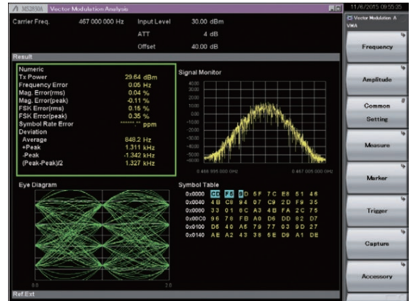
4FSK Modulation Analysis Measurement Example
