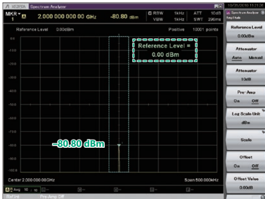
Example: Level Stability by Switching Reference Level
