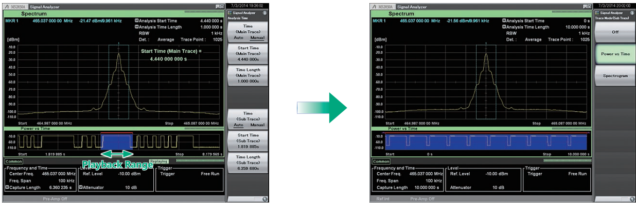
Playback any Desired Section of Captured Waveform
